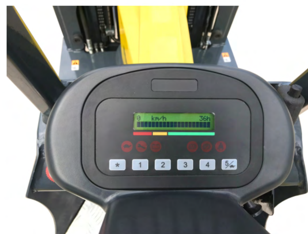
ZAPI dashboard displays failure codes
