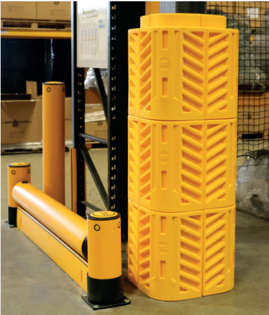
Stepped stacking feature connects multiple Column Protectors together so they act as one integrated unit instead of separate systems. The step enables the stacked assembly to lock in place and allows energy to transfer throughout the entire system for even greater protection at increased heights.
